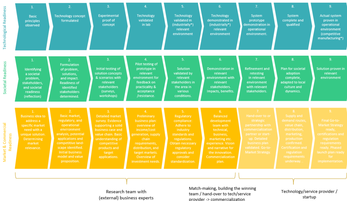
Figure 2. Technological 1 , societal 2 and market & commercial readiness 3 assessment scales. Ideally, all three readiness scales advance approximately side by side in the innovation process. In practice, each innovation is different with a unique pathway to market, technological, and societal readiness.
